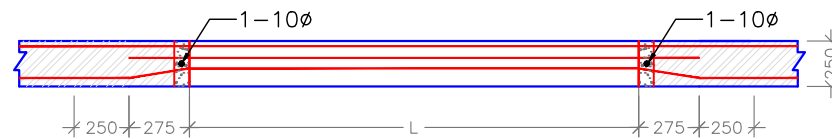
BOTTOM REINFORCEMENT LAYOUT PLAN
